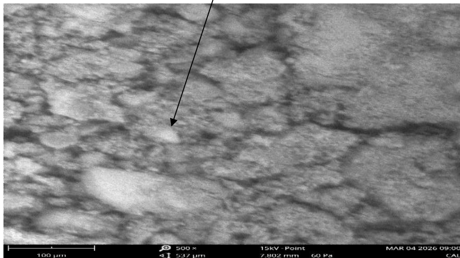
Plate III: SEM Image of Pore Structure of Precipitated Calcite
