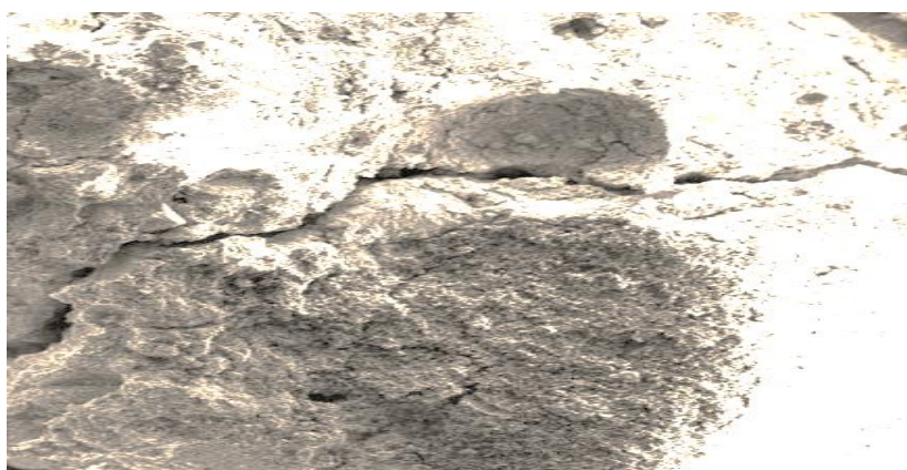
Plate II: SEM Image of Pore Structure of Mk-NSA Concrete (5% Mk - 5% NSA)
